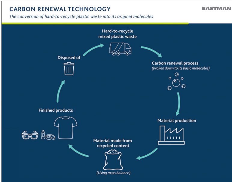
Eastman molecular recycling technologies (Polyester Renewal Technology and Carbon Renewal Technology) span a range of eyewear plastic materials.
