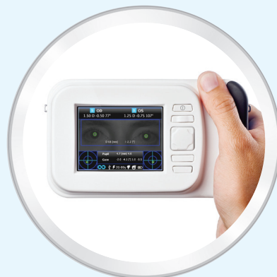
The compact, lightweight 2Win Refractometer is fully automated, runs on batteries and offers printer and PC connectivity.
