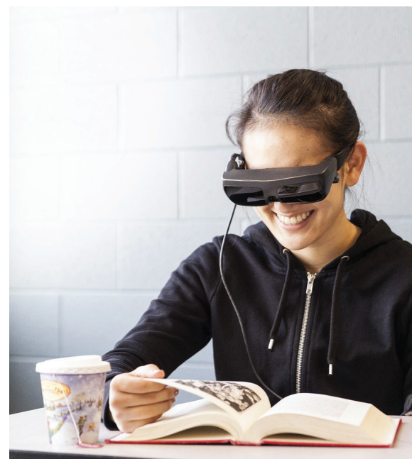
eSight eyewear delivers real-time video images which users can enhance, magnify and adjust to ensure their eyes can best interpret their surroundings.
